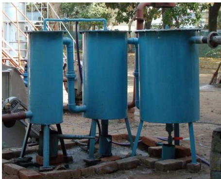
Fig 3.2 Wetbed scrubber with raschig rings, charcoal and coconut coir (from left to right)
